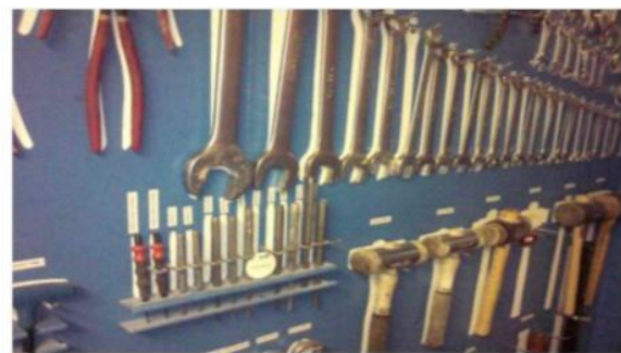
Fig 2: Shadow Board Displaying all the Equipment and tools at its Right Place
